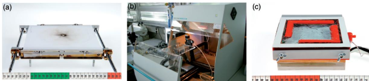
FIG. 1—Two sample holders and the sample chamber of the millimeter-X-ray fluorescence analysis (m-XRF) Spectro *Midex M*—(a) Clamp frame for the investigation of gunshot residue (GSR) on fabrics and adhesive tapes, (b) Spectro *Midex M*: sample chamber, (c) Peltier-cooled sample holder for the investigation of GSR on tissues.
